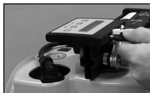
Figure 10: Connect Transformer Power Cord
